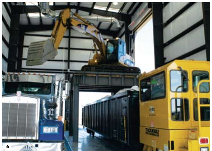
6 high-throughput emission controlled railcar unloading
