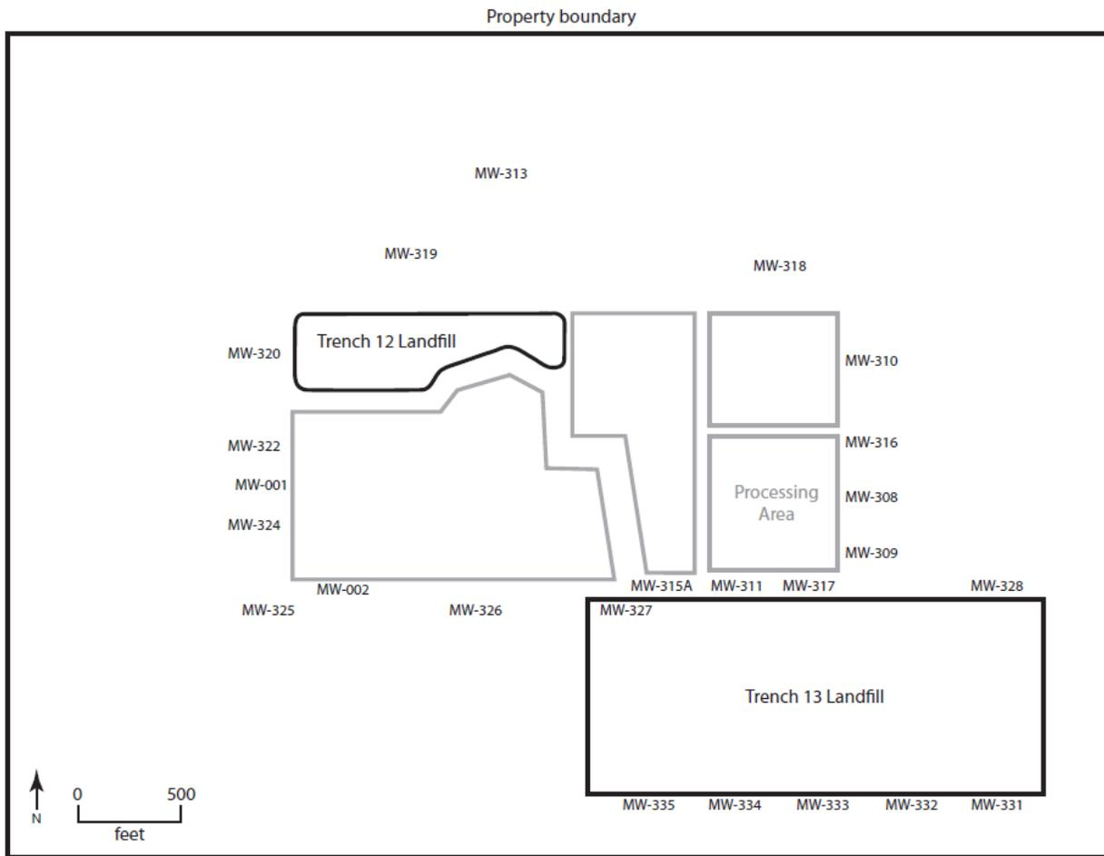
Figure 3. Groundwater Monitoring Wells, US Ecology Nevada
